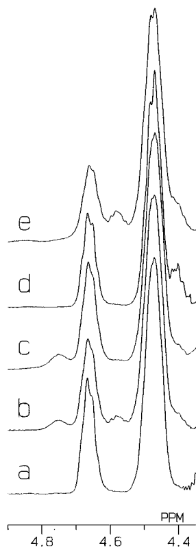
Figure 6. ^1\text{H} NMR spectra of sodium polyaspartate and model polymers measured at 80 °C and pD 8 in \text{D}_2\text{O} : (a) high molecular weight SPA-2; (b) SPA-1 thermally prepared without phosphoric acid catalyst; (c) SPA-6 with many laurylamide branched units; (d) SPA-4 with many \alpha and \beta -dicarboxylic acid end groups; (e) SPA-3 with many asparagine end groups.
